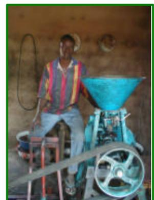
The mill, coupled to the engine for agricultural production
