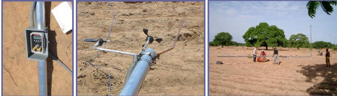
Data recording box (left); The Sensor of wind direction and the anemometer (middle); Assembling of the Gin-pole (right).
