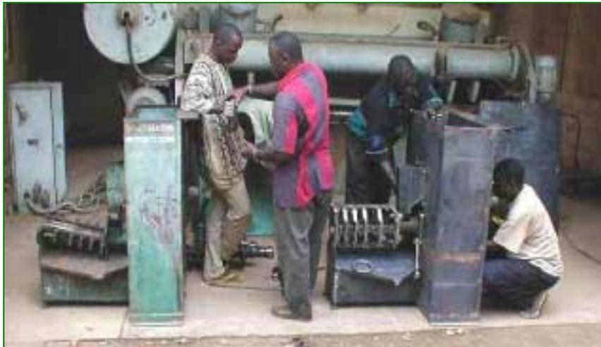
Technology transfer South-South within the framework of project SEAF I, the press on the left is an original 'Sundhara' press, which comes from Nepal. On right-hand side is the new Malian press. These presses are used for the extraction of jatropha oil. MFC, SEAF I
