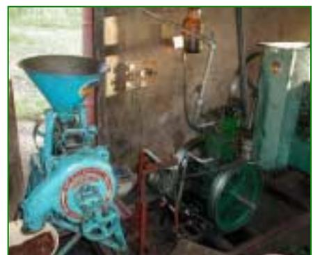
A multipurpose platform using jatropha oil as fuel. The installations of N'Tjila (Sikasso) and Falan (Koulikoro), were rehabilitated by MFC within the framework of the SEAF I project.
