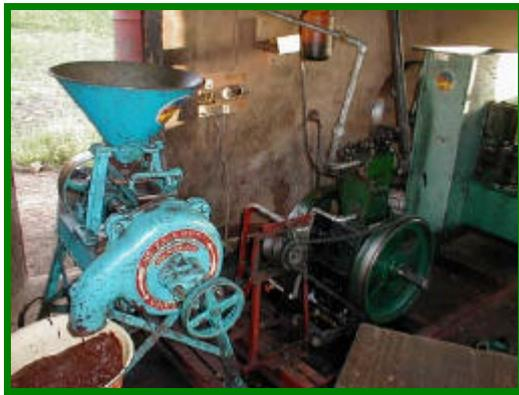
The mill for grinding Shea nuts (left), the battery charger (adjacent), the motor (centre) and the jatropa press (far right)
