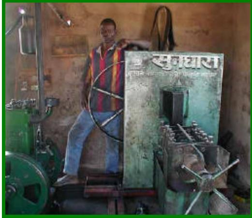
**The operator with the plant oil engine (left) and the press (right).**
