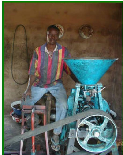
Mill for grinding Shea nuts.
